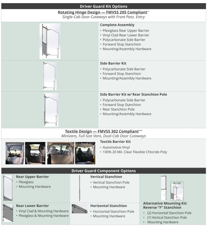
\*\*Our polycarbonate side/center barriers are superior to plexiglass and AS-4 certified, meeting FMVSS 205 requirements. \*\*\*Our textile barrier materials meet the Federal Motor Vehicle Safety Standard No. 302 (FMVSS 302) which specifies the burn resistance requirements for materials used in the occupant compartments of motor vehicles.
